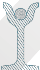
Sheave groove matches rope
