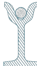
New rope will be damaged
