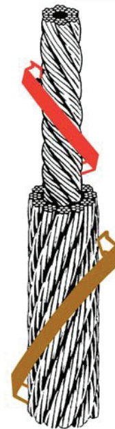
Example of a 2-layer rotation resistant construction with 12 outer strands. (19x7)
