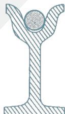
Sheave groove too small
